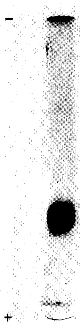
Fig. 3. Disc electrophoresis of purified beef brain ribonuclease. (A) Densitometric profile of analytical polyacrylamide gel of purified beef brain RNAase. Purified RNAase, 5 \mu g obtained after chromatography on Sephadex G-100 superfine was applied on two identical 10% polyacrylamide gels in \beta -alanine/acetic acid buffer (pH 4.5). Electrophoresis was carried out for 6 h at 0.4 mA/gel. In the extract of slices of the unstained gel RNAase activity was found to coincide with the unique band. The arrow indicates the position of cytochrome c. (B) Resolution of purified beef brain RNAase by gel electrophoresis on a 10% polyacrylamide gel (pH 7) containing 0.1% sodium dodecylsulphate [19]. Purified beef brain RNAase was heated for 2 min at 100°C in the presence of 0.1% sodium dodecylsulphate and 0.1% \beta -mercaptoethanol before electrophoresis. 6 \mu g of protein was applied to the gel.
